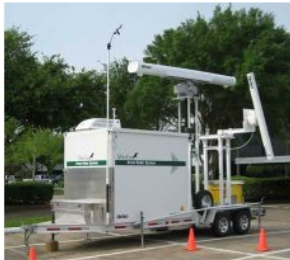
Figure 7: Advanced avian radar system developed by DeTect, Inc. of Panama City, Florida, model MERLIN XS2530e
