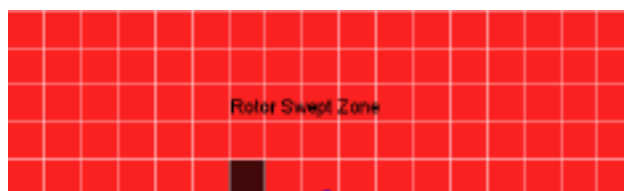
Figure 11: Array of discrete pathways in the rotor swept zone with one of all the Discrete Pathways blocked by a wind turbine
