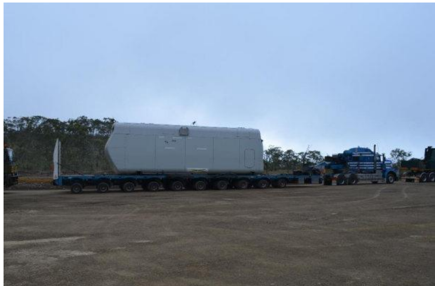
Nacelle delivery to upper compound
